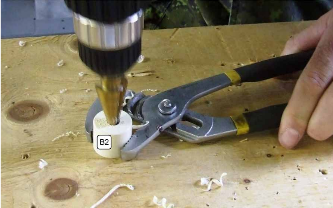
Figure 11-A Section B, Drilling the hole for the tire valve stem.
