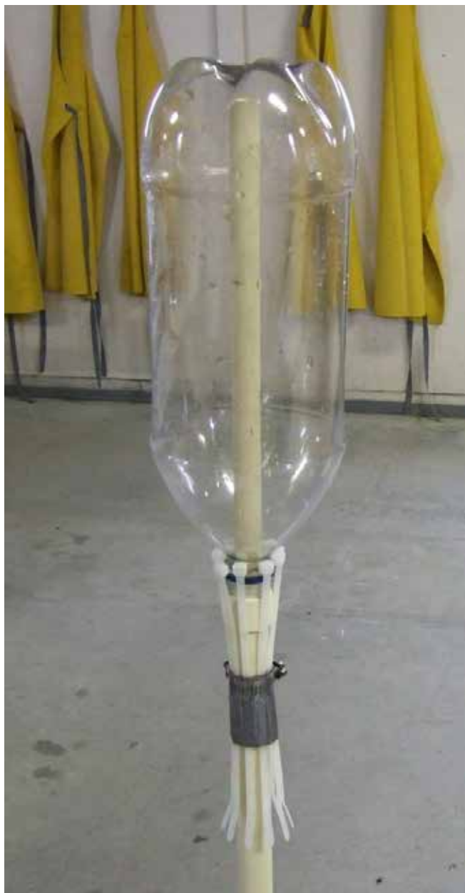
Figure 24-A Cable Ties Holding the Soda Bottle
