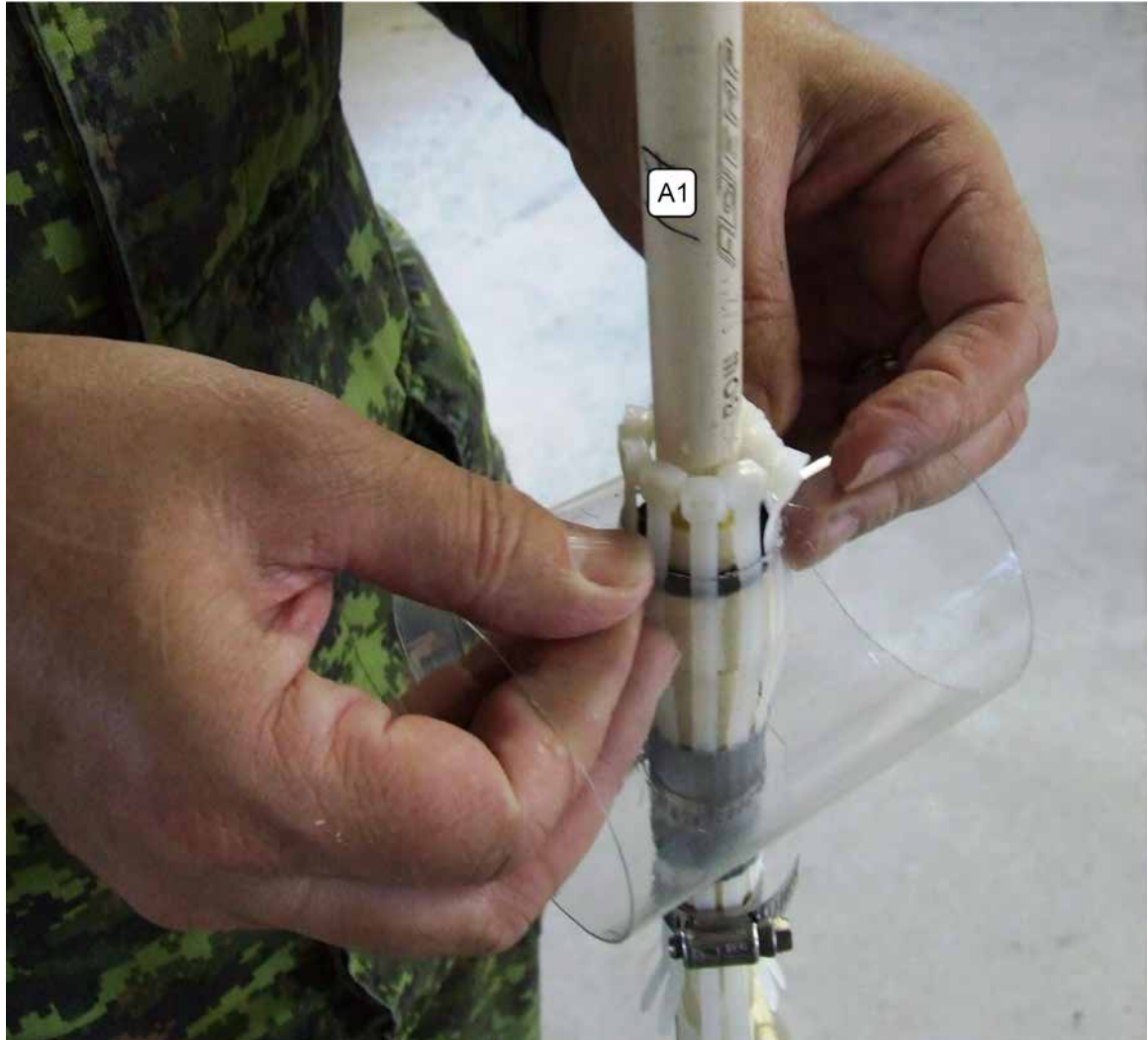
Figure 28-A Sliding the Spring over the Cable Ties
